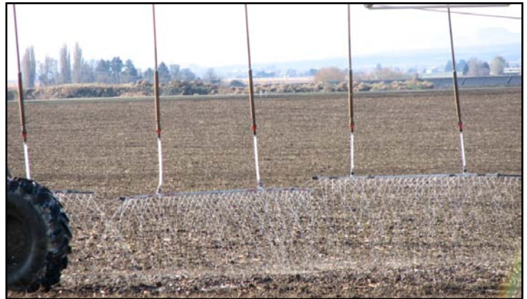
A drizzle boom-type system fitted to the drop tubes of a center pivot.
