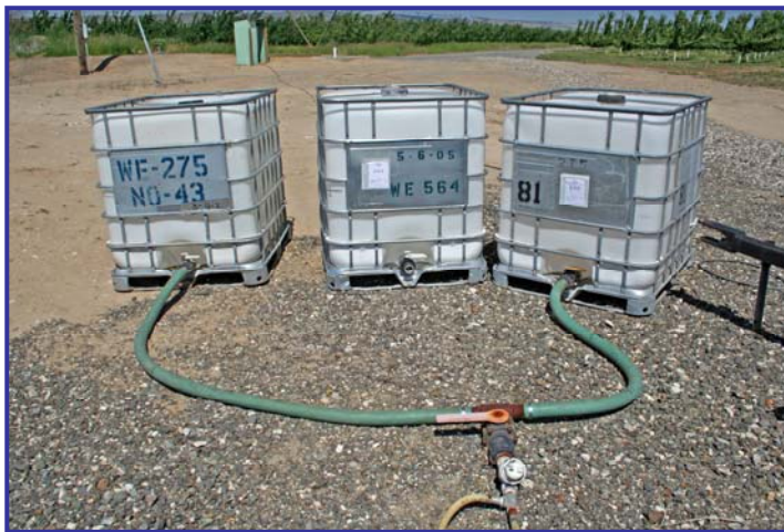
Figure 7. Identification information must appear on each mini-bulk container, even if the containers are manifolded together.
