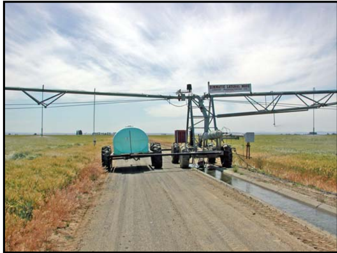
Figure 2. Linear (or lateral) move irrigation system.
