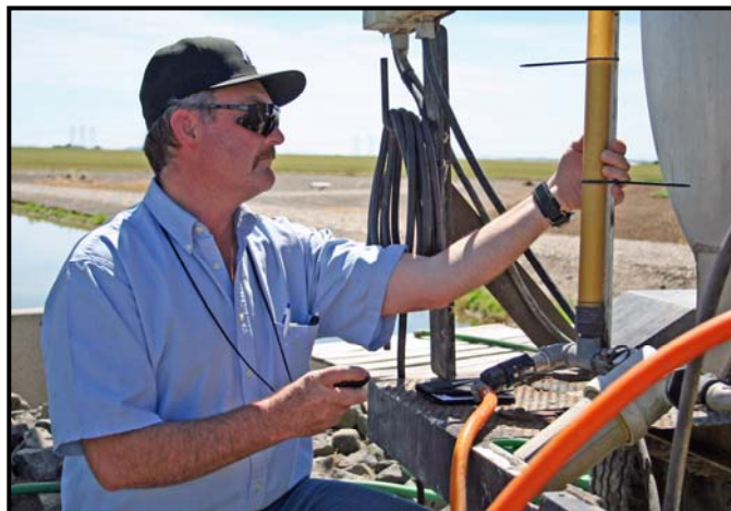
Figure 3. Throughout an application, the injection system should be periodically recalibrated to verify the application rate.
