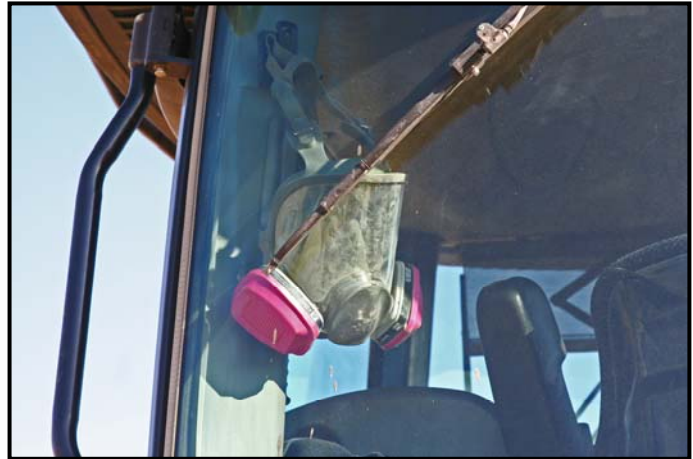
Figure 8. A respirator must be worn while in a tractor cab if the pesticide label requires an applicator to wear a respirator.
