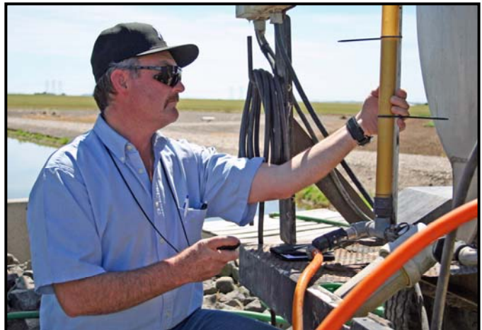
Figure 3. Throughout an application, the injection system should be periodically recalibrated to verify the application rate.
